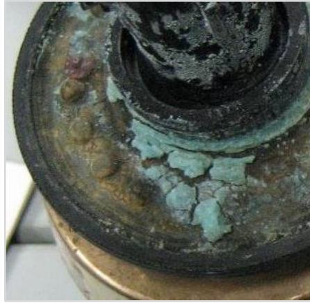
Debris blocking diaphragm
