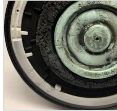
Degraded relief valve disc
