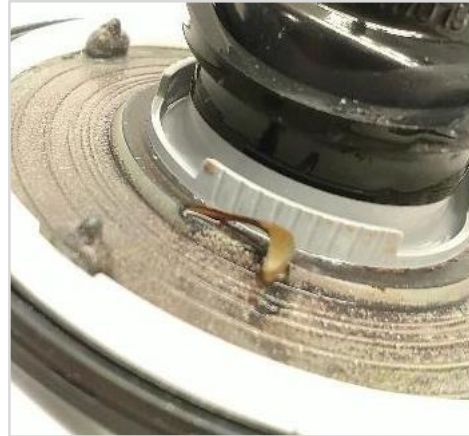
Debris under diaphragm
