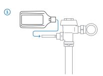
① No adjustments needed. Slide the handle mount over the existing flushometer handle and tighten.
