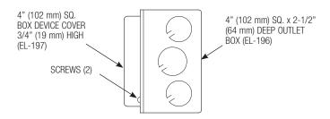
Install Electrical Box into Wall Box as follows
