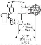
‡ IMPORTANT: IF INSTALLED AT MAXIMUM DISTANCE, STOP MAY INTERFERE WITH WALL BOX FRAME.
