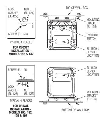
Install Wall Box into wall in the exact location as illustrated in the Rough-in diagrams on Pages 2 and 3. Secure Wall Box using Drive Screws provided or other appropriate fasteners.
