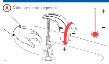
Optional — To fix temperature, set lever to the desired position, then remove lever and plug hole with Cap.
