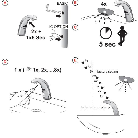
**DISCLAIMER:** Updated electronics have visible red and green LED. Original electronics have only red LED and range setting is reversed (1=longest, 8=shortest).
