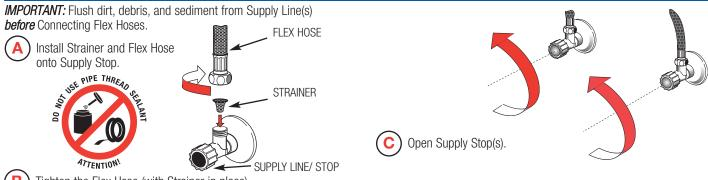
B Tighten the Flex Hose (with Strainer in place) securely to the Supply.
