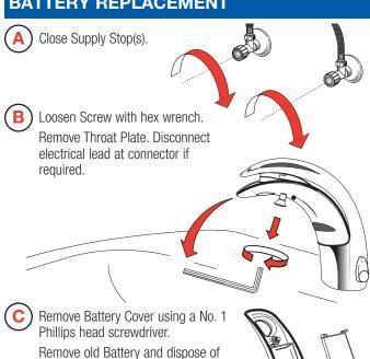
Insert a new 6 Volt Type 2CR5 Lithium Battery. The red LED will flash for one (1) minute.
