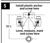
Measure and mark rough in. Use a 5/16" masonry bit to drill hole, then install the hanger bracket with one plastic anchor and screw. Level the bracket then mark, drill and install two plastic anchors and screws.
