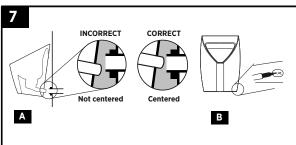
**A. Hang bowl on the bracket** and check tail pipe alignment, then remove the bowl and adjust the bracket as needed. Re-hang and re-check bowl alignment with the drain line. Tail pipe should align with center of drain line.
