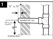
Set drain line height 17" from finished floor (standard 24" rim) or 10" for ADA installation. Threaded nipple should extend 1/2 to 3/4" from wall. \*IMPORTANT Nipple must not extend more than 3/4" past the finished wall
