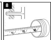
**Determine the drain nipple length** by measuring the distance between the back of the sanitary tee (or elbow) to the front edge of the nipple.
