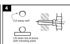
**Adjust drain to achieve pitch** only if standing water is present (code requires 1/4" drop per foot of drain line for proper pitch). Seal wall according to code.
