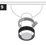
PLACE THE HOSE CLAMP and compression nut onto the housing tailpipe.
