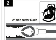
**IMPORTANT:** Use a drain machine to remove build-up inside pipes. Clean up to 25 feet deep then flush with water to remove cutting debris. Never install on copper DWV.
