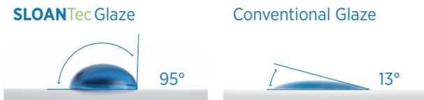
To ensure the unique hydrophobic and oleophobic properties of SloanTec glaze were permanent and could stand up to the harsh conditions in commercial restrooms, we conducted a series of tests to artificially age the surface.
