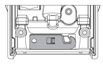
C Insert spray removal tool into spray slot by sliding hook end of key between faucet spout and insert. Pull insert out of faucet once hooked.
