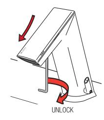
**(B)** Place new crown on faucet by sliding onto spout and tightening hex screw on underside of spout.
