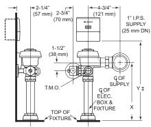
X MODEL 110/111 - 11½" (292 mm) Y MODEL 110/111 - 19" (356 mm) MODEL 113 - 16" (406 mm) MODEL 113 - 19" (483 mm)
