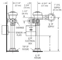
X MODEL 115 - 24" ‡ (610 mm) Y MODEL 115 - 14" ‡ (356 mm) MODEL 116 - 27" ‡ (686 mm) MODEL 116 - 17" ‡ (432 mm)
