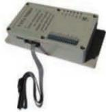
Vata Verks Smart Sensor detects the mechanical movement within the utility meter when flow occurs, and converts that movement to
