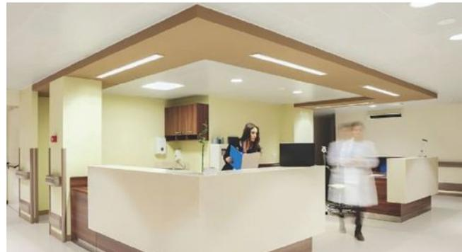
**Ecore's** newest commercial surface, **Aurora**, is a resilient rubber sheet that features a polyurethane-coated (PUR-coated), calendared-rubber wear layer that is fusion-bonded to an Ecore vulcanized composition rubber (VCR) backing. The result is flooring that provides enhanced ergonomics, comfort, and safety for healthcare workers, visitors, and patients. The surface is hygienic due to a heat-welded installation process.
