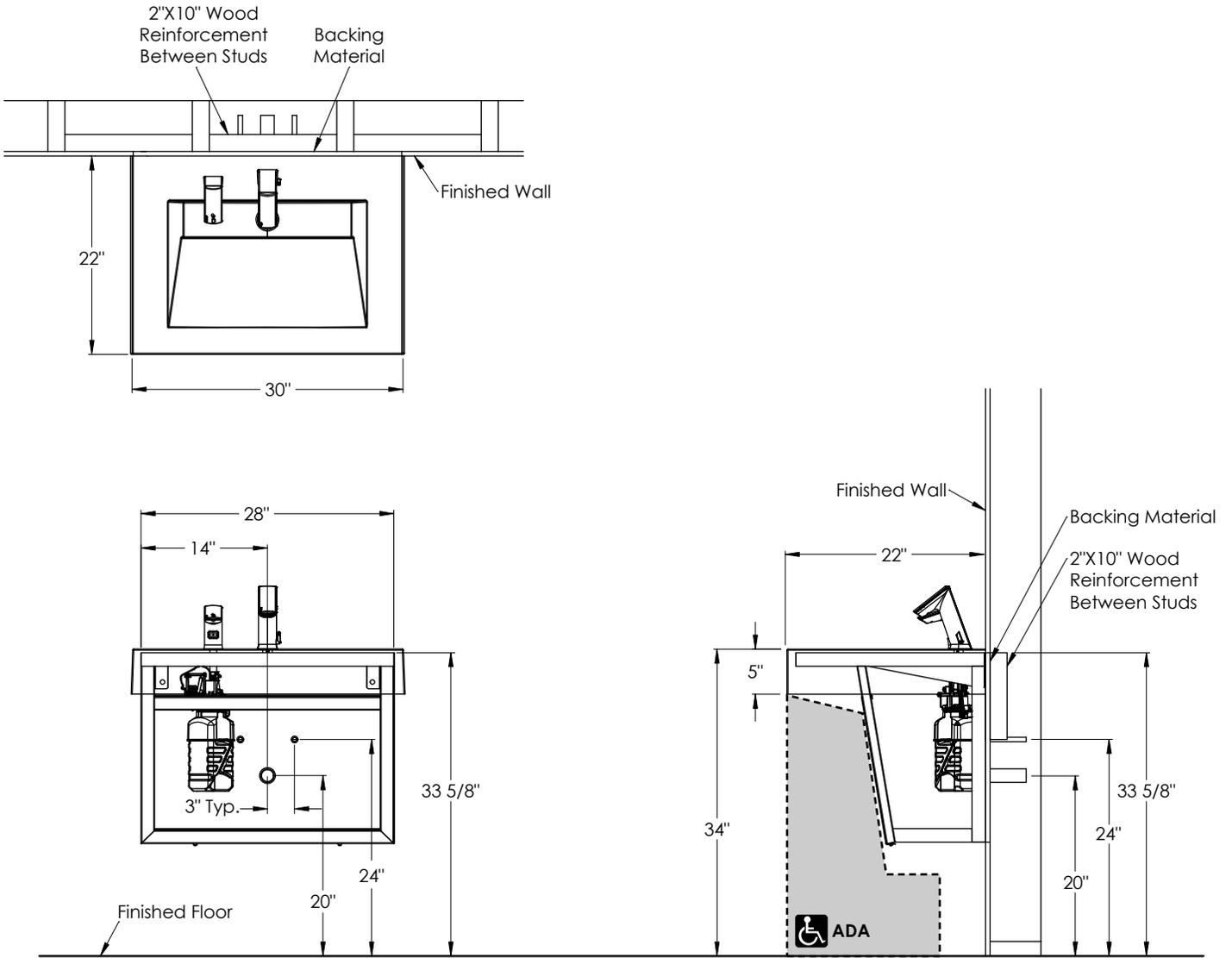
**Note:** Backing material should equal thickness of drywall, 1/2" min.
