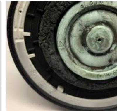
Degraded diaphragm assembly
