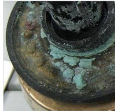
Debris blocking diaphragm bypass
