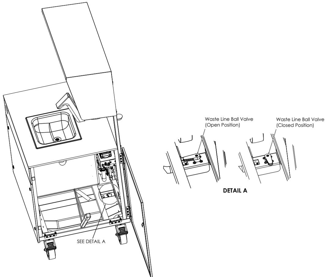
1. Drain the waste tank (Gravity Fed).
