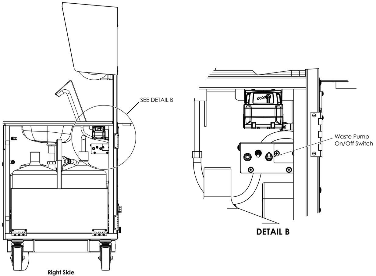
1. Drain the waste tank (Electric Pump).
