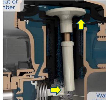
Plunger tilts the relief valve, causing diaphragm to unseat and flush begins
