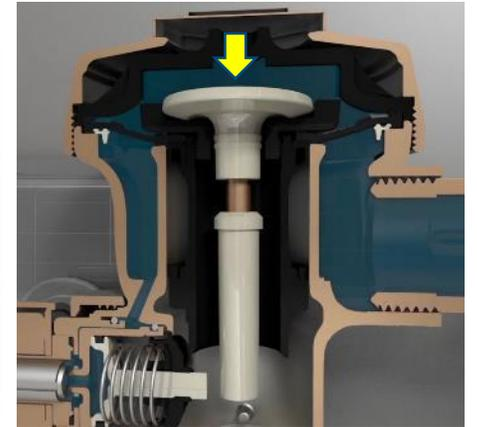
Upper chamber re-pressurizes through the bypass, causing diaphragm to re-seat and ending flush
