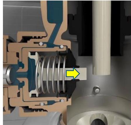
Solenoid movement permits water to flow into actuator cartridge and pushes plunger forward
