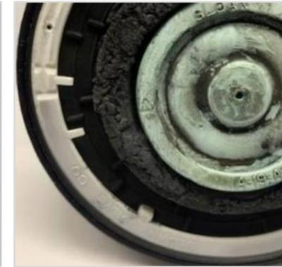
Degraded diaphragm assembly
