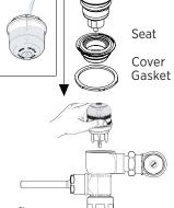
• Insert inner cover gasket flat into the body (below the cover threads)
