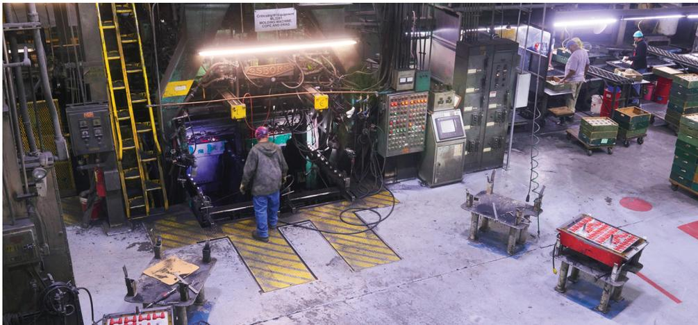
*Sloan's Osborn inline tight flask is 30" x 22" x 7"/7" and operates at 250 molds per hour. Each mold has two patterns of 21.5" x 14.7". The casting production of a one pound tail casting is 12,000 pieces per hour.*
