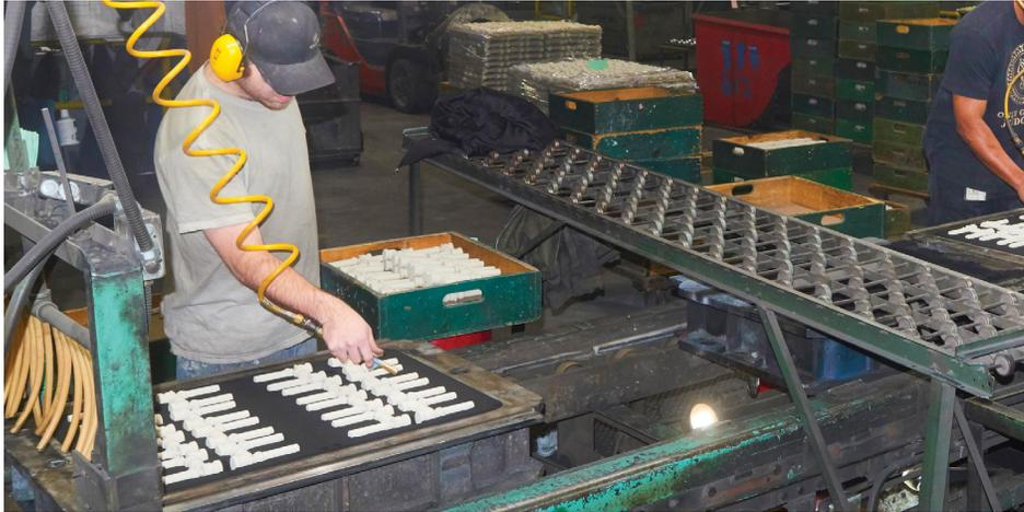
*Multiple core setting stations allow for 250 mold per hour production while setting numerous cores.*
