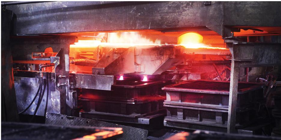
*Auto pour unit provides uniform pouring parameters for each casting by controlling metal temperature and pouring rate for each unique casting.*
