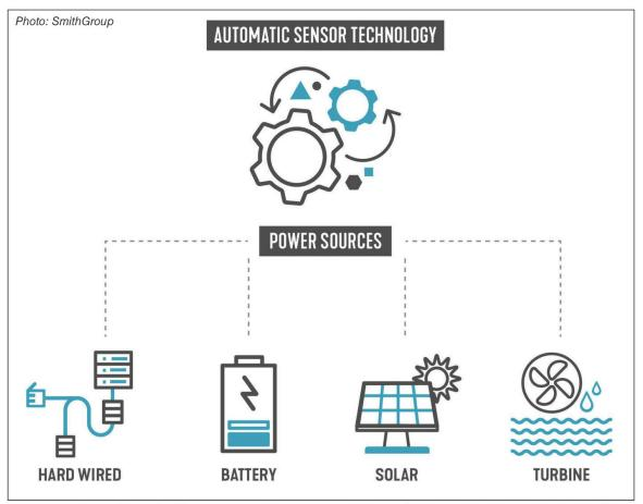
but on a much smaller scale. The movement of water through the unit spins a turbine that generates electricity to supplement battery usage.
