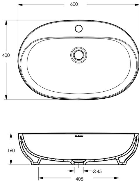
**Note:-**All vitreous china dimensions shown in these drawings are nominal. Dimensions can vary within the tolerances established in the governing BIS standard. Please take this into consideration when planning rough-in and plumbing layouts. Product illustrations shown are representative only; actual products may vary. Sloan reserves the right to make changes in product characteristics, packaging or availability at any time without notice.
