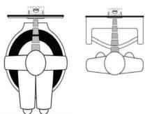
When the user steps away, the sensor initiates a "one-time" signal that activates the flushing cycle to flush the fixture (1 second delay for urinal, 3 seconds delay for closet). The Circuit automatically resets and is ready for the next user.
