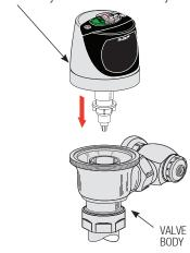
To facilitate installation, the 0-ring on the diaphragm assembly must be wet for easier insertion. NOTE: Sensor Lens must face directly forward. Rotating the Sensor to either side will decrease the Sensor's ability to detect a target.
