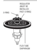
Optima Plus Valve Models Feature Sloan's Exclusive Flex Tube Diaphragm<sup>™</sup> for the ultimate in valve performance, reliability and Chloramine resistance.
