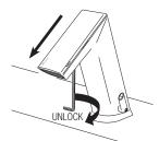
Place new crown on faucet by sliding onto spout and tightening hex screw on underside of spout.
