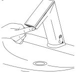
Cover IR clic until LED flashes 4x - hold until LED flashes 1x to 8x, from minimum to maximum. See diagram below. Release when requested range is reached.
