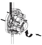
Remove filter from solenoid caddy assembly.
