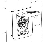
7. Rotate the button 90° back to lock it in place.
