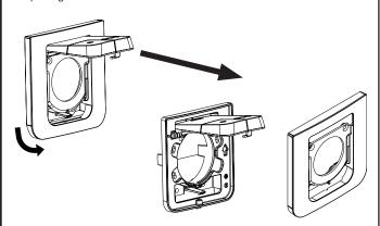
**3.** Mount the Wall Bracket to valve and secure it using the Bracket to Valve Screws (supplied).
