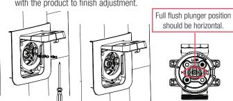
**6.** Using the depth tool (supplied), adjust depth of plunger screws until screws touch depth guide (use provided alternate length screws if necessary), hold screw and secure nuts against plunger.
