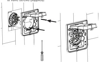
**4.** Mount the Face Plate on the black Wall Bracket and secure it using the Plate to Valve Screws (supplied).
