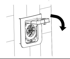
**8.** Test flush by pushing button (make sure that button is not pushing the screws when not being pressed).
