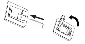
2. Remove the face plate by tilting it up from the bottom and then pulling it out.
