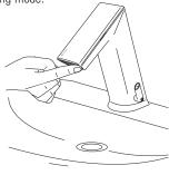
Cover IR clic until LED flashes 4x - hold until LED flashes 1x to 8x, from minimum to maximum. See diagram below. Release when requested range is reached.
