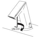
Retrieve spray removal tool located near the spray insert.
