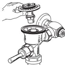
**C** Reinstall Outside and Inside Cover wrench tight. Open Control Stop to flush supply line. Close Control Stop and remove Outside and Inside Cover.
