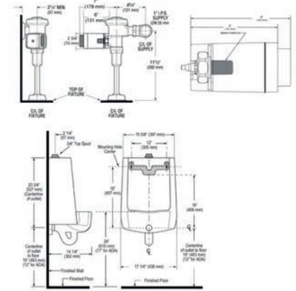
NOTE: Allow extra for height requirements above all heights 17" and below. Allow extra for mounting height to the floor to achieve a 600" min height or more in shower compartments.
