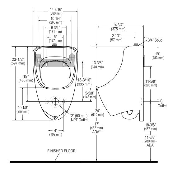
NOTE: ADA urinal rim height requirements allow all heights 17" and below. Sloan strongly recommends roughing in the drain to achieve a 16<sup>1</sup>/<sub>2</sub>" rim height or less to ensure compliance.
