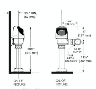
Alternate ADA Installation Lower water supply rough-in to 10" (254 mm) and mount grab bar at the 36" (914 mm) maximum allowed height.
