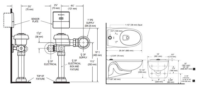
+ Position of Sensor Box can be raised or lowered 1" (25 mm) if in conflict with Handicap Grab Bars.
