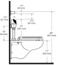
WHEN INSTALLING IN A HANDICAP STALL: Per the ADA Guildlines (section 604.9.4) it is recommended that the grab bars be split or shifted to the wide side of the stall. If grab bars must be present over the valve,
