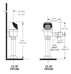
When installing the Flushometer in an ADA compliant stall:
