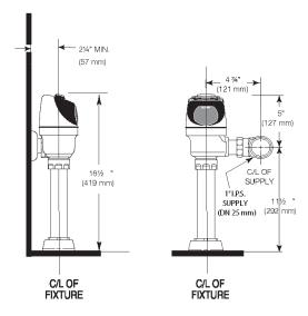
When installing the Flushometer in an ADA compliant stall:
