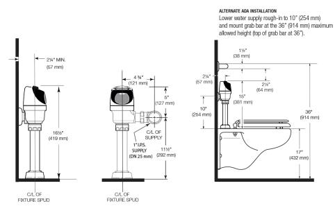
WHEN INSTALLING IN A HANDICAP STALL: Per the ADA Guildlines (section 604.9.4) it is recommended that the grab bars be split or shifted to the wide side of the stall. If grab bars must be present over the valve, use the alternate ADA installation as shown to the right.
