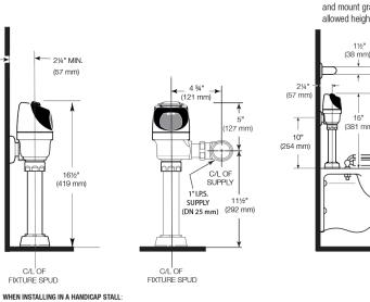
Lower water supply rough-in to 10" (254 mm) and mount grab bar at the 36" (914 mm) maximum allowed height (top of grab bar at 36").
