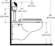
WHEN INSTALLING IN A HANDICAP STALL: Per the ADA Guildlines (section 604.9.4) it is recommended that the grab bars be split or shifted to the wide side of the stall. If grab bars must be present over the valve, use the alternate ADA installation as shown to the right.
