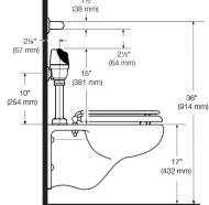
WHEN INSTALLING IN A HANDICAP STALL: Per the ADA Guildlines (section 604.9.4) it is recommended that the grab bars be split or shifted to the wide side of the stall. If grab bars must be present over the valve, use the alternate ADA installation as shown to the right.
