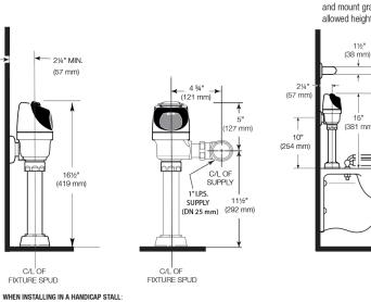
ALTERNATE ADA INSTALLATION Lower water supply rough-in to 10" (254 mm) and mount grab bar at the 36" (914 mm) maximum allowed height (top of grab bar at 36").
