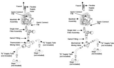
SINGLE INLET FILTER FITTING KIT WITH BELOW DECK THERMOSTATIC MIXING VALVE (BDT)
