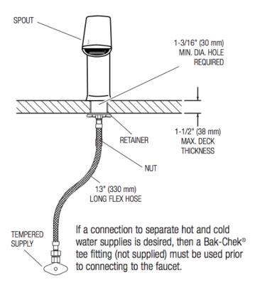
Thermostatic mixer ordered separately to comply with ASSE 1070 requirements. The product shall be tested and certified to industry standards: ASME A112.18.1M, CSA B125.1, California Health and Safety Code 116875
