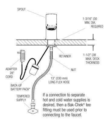
supply upon removal eliminating, need to access control stops. Solenoid carrier includes strainer for easy above deck service. Thermostatic mixer ordered separately to comply with ASSE 1070 requirements. The product shall be tested and certified to industry standards: ASME A112.18.1M, CSA B125.1, California Health and Safety Code 116875
