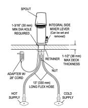
**Electrical Connection for up to 6 Faucets** Can combine up to six (6) faucets using one adapter
