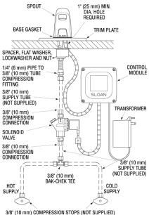
ETF-610 Faucet with ADM Variation Mixing Valve for Hot and Cold Water Supply (shown with 8" trim plate)
