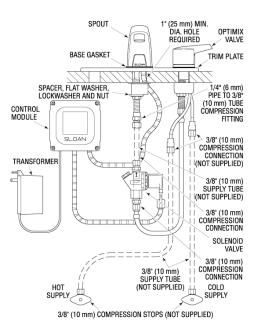
ETF-610 Faucet with BDM and BDT Variation Mixing Valves for Hot and Cold Water Supply (shown with 4" trim plate)
