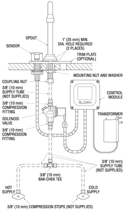
ETF-770 Faucet with ADM Variation Mixing Valve for Hot and Cold Water Supply (shown with 4" trim plate)
