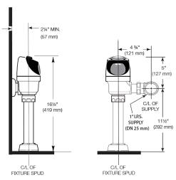
Lower water supply rough-in to 10" (254 mm) and mount grab bar at the 36" (914 mm) maximum allowed height (top of grab bar at 36").
