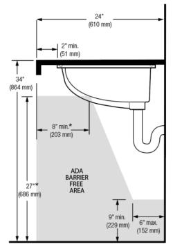
\*The dip of the overflow shall not be considered in determining knee and toe clearance (2010 Federal ADA, ANSI A117.1, TAS)
