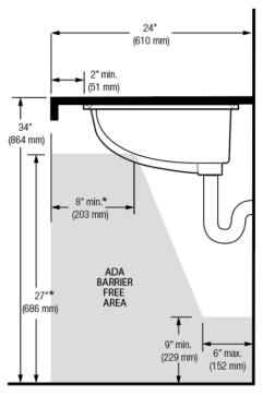
\*The dip of the overflow shall not be considered in determining knee and toe clearance (2010 Federal ADA, ANSI A117.1, TAS)
