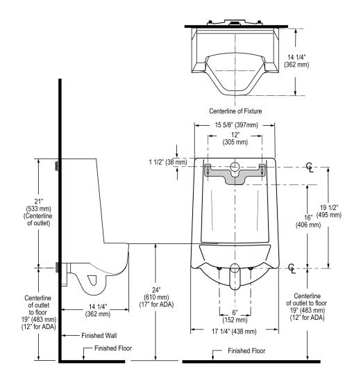
NOTE: ADA urinal rim height requirements allow all heights 17" and below. Sloan strongly recommends roughing in the drain to achieve a 16<sup>1</sup>/<sub>2</sub>" rim height or less to ensure compliance.
